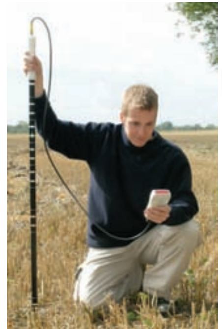
(Above) PR2/6 Profile Probe with HH2 Moisture Meter. (Right) PR2/4 Profile Probe
