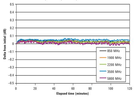
Repeatability measures the ability of the instrument to return to a given power setting after a random excursion to any other frequency and power setting. It should not be confused with absolute level accuracy.
