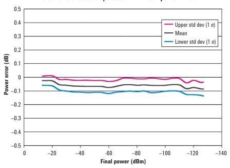
Relative level accuracy measures the accuracy of a step change from any power level to any other power level. This is useful for large changes (i.e. 5 dB steps).
