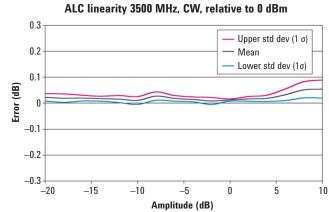
Linearity measures the accuracy of small changes while the attenuator is held in a steady state. This is useful for fine resolution changes.
