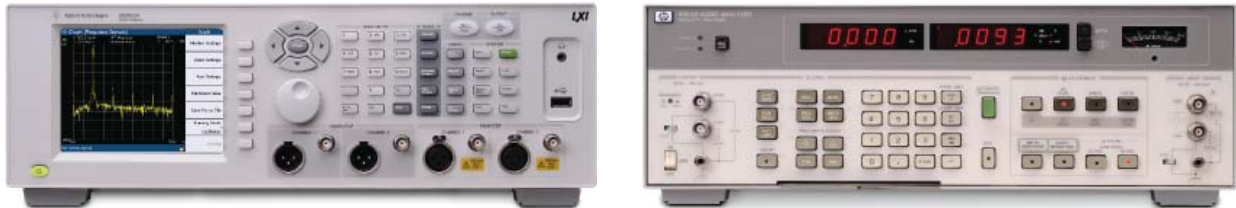
Figure 1. The new U8903A audio analyzer (left) offers numerous improvements over the widely used HP 8903B (right).
